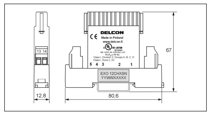
EXO 12CHXSN (dimensions in mm, nominal). Markings can be located differently by production lot. Parts of the markings are backside of the relay. Production lot number is marked to the socket (YY = year, WW = week, XXXXX = lot number).
