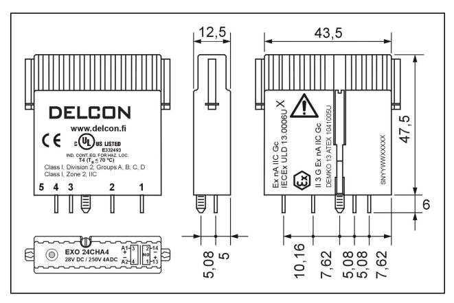
EXI 24CHA4 (dimensions in mm, nominal). Markings can be located differently by production lot. Production lot number is marked to the relay (SN = serial number YY = year, WW = week, XXXXX = lot number).
